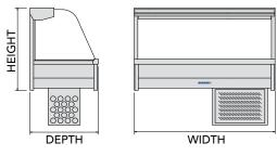
Note: For overall height dimensions, add height of motor cage (450 mm).
