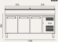
Allow min. 100mm clearance for instalation,
